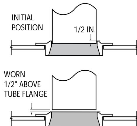
*Feed tube placement within 1/2 inch of the top of the tube flange for SuperChipper™ Rotors*
