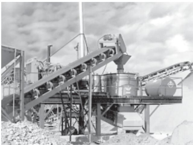
*Frame mounted on a concrete slab*
