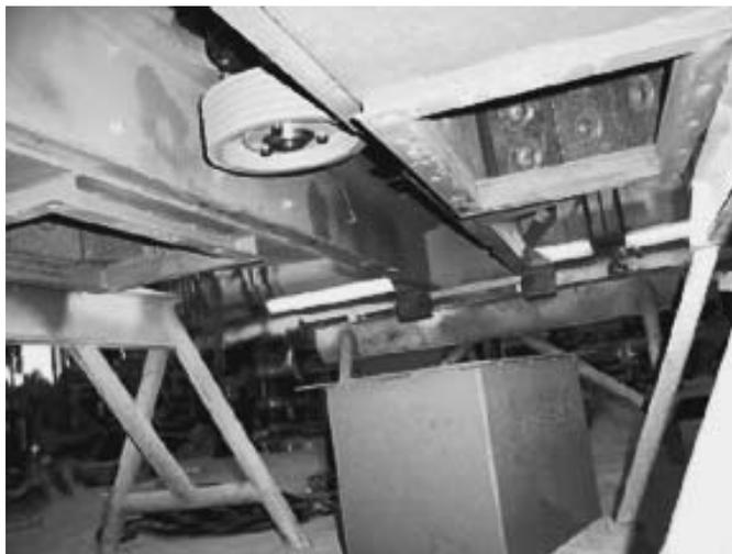
*Standard discharge chute ready for installation*
